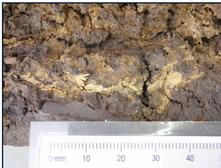
Figure 1. Jarosite in a soil core from far north Queensland. The yellow mineral is soft to touch.
