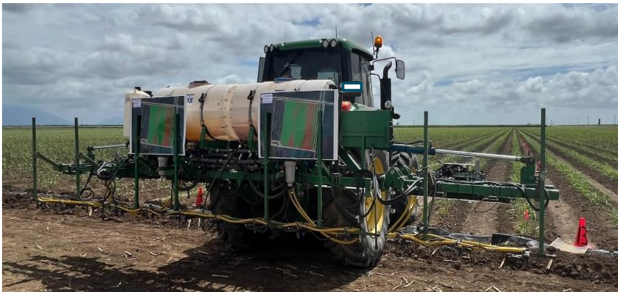
Image 1 AutoWeed experimental dual-tank herbicide spray rig at a Field Day demonstration in the Burdekin region and displays of example trial spray application maps
