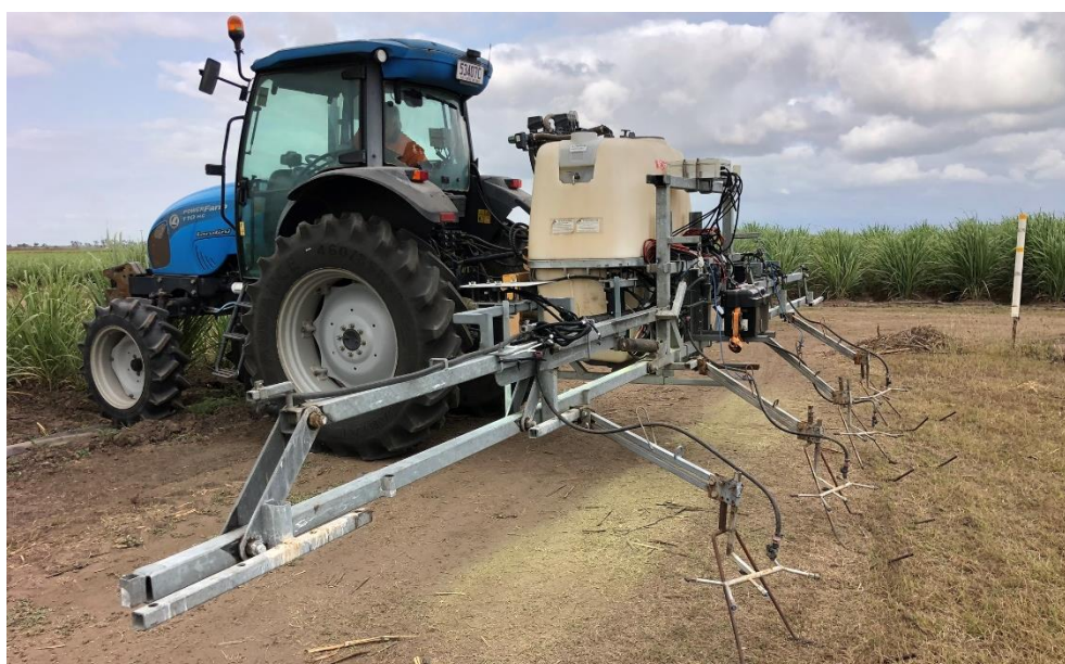
Image 3 Tractor fitted with AutoWeed spraying units during a project trial. Image used with permission. Copyright © 2023, AutoWeed. All rights reserved.
