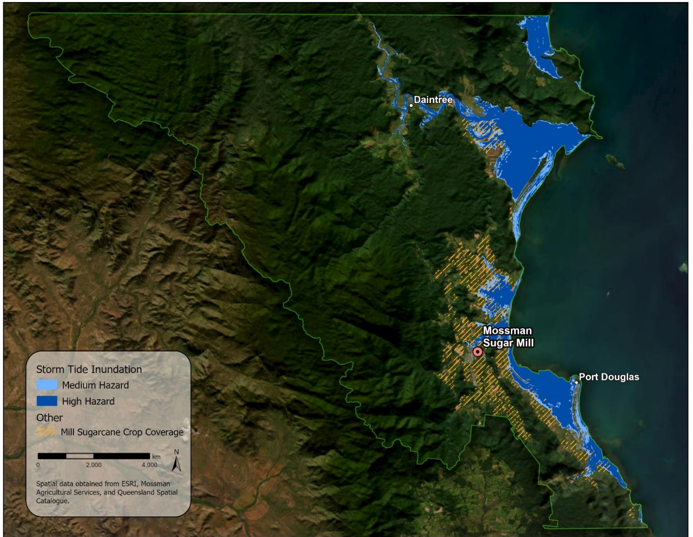
Figure 6: Storm tide hazard maps of the Mossman District, based on Queensland Government 'Storm Tide High Hazard Queensland' and 'Storm Tide Medium Hazard Queensland' products, including projected sea level rise (+0.8 m) as a result of climate change by 2100. The medium and high hazard areas refer to areas inundated by less than and greater than 1 metre of water, respectively. This map is created from Version 4 of the Storm Tide Inundation Area products of The State of Queensland Department of Environment and Science (State of Queensland Department of Resources, 2022).
