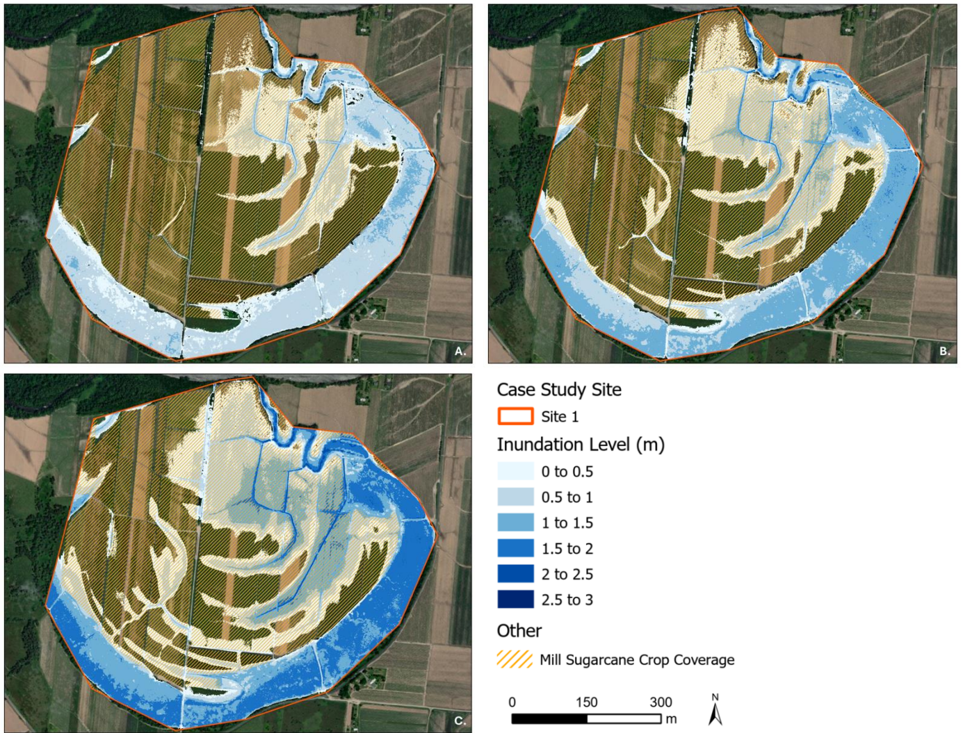
Figure 26: Inundation levels of case study site 1 under the current highest astronomical tide (HAT) (A.), as well as inundation by year 2057 (B.) and 2107 (C.) due to climate change. Boundaries were generalised for modelling and resulting inundation was reduced to the boundary to highlight inundated areas specific to the site. Mill crop coverage data provided by the Mossman Agricultural Services.
