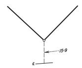
Railway centre lines—connections to 'Rly' are to be shown either on face or by tabulation in the 'Traverses etc.' table.
