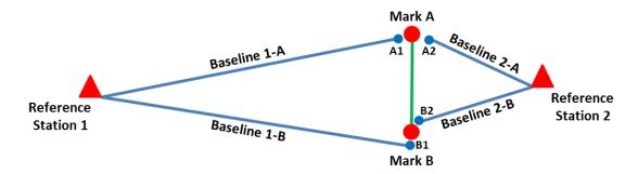
In the following calculations, it is assumed that the two reference stations have been surveyed to a high quality (e.g. are existing GDA Datum PSMs) such that any relative uncertainty between them has minimal effect when comparing A1 to A2 or B1 to B2.
