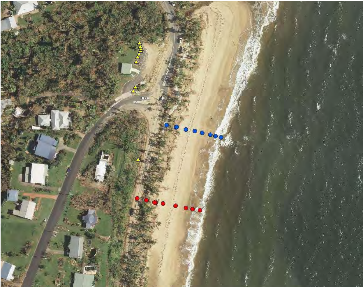
Figure 20: Bingil Bay surveyed beach profiles and debris lines (yellow triangles)
