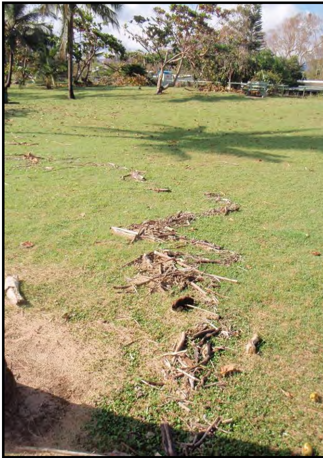
Photograph 41: Debris line used to survey storm tide inundation level (Source: DSITIA)
