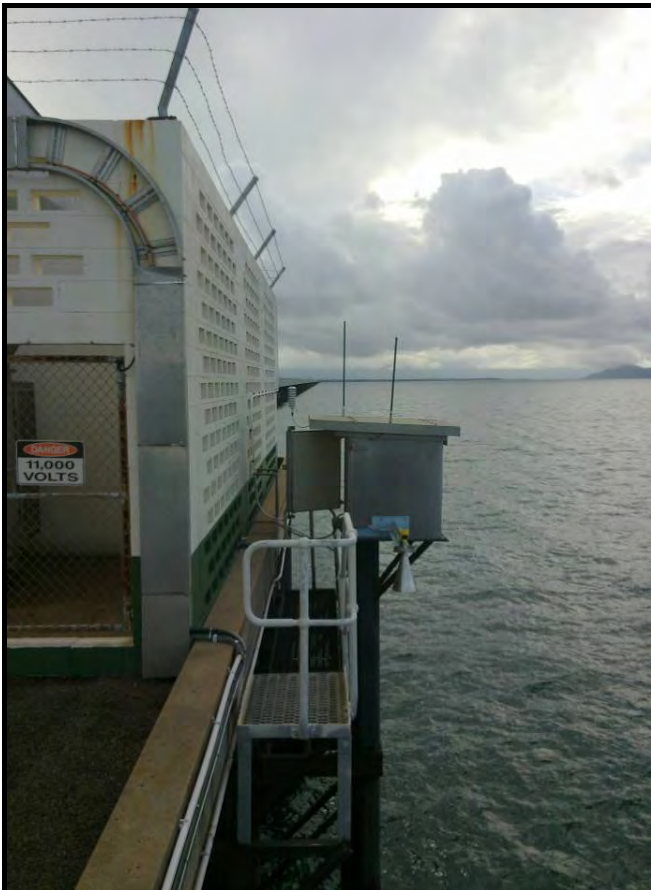
Photograph 32: DSITIA's offshore storm tide gauge at Lucinda prior to TC Yasi (Source: DSITIA)
