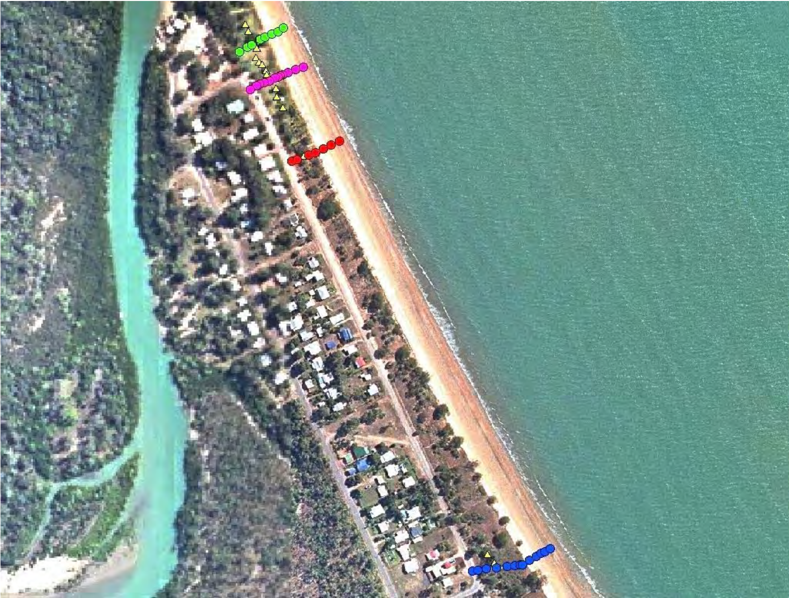
Figure 36: Balgal Beach surveyed beach profiles and debris lines (yellow triangles)
