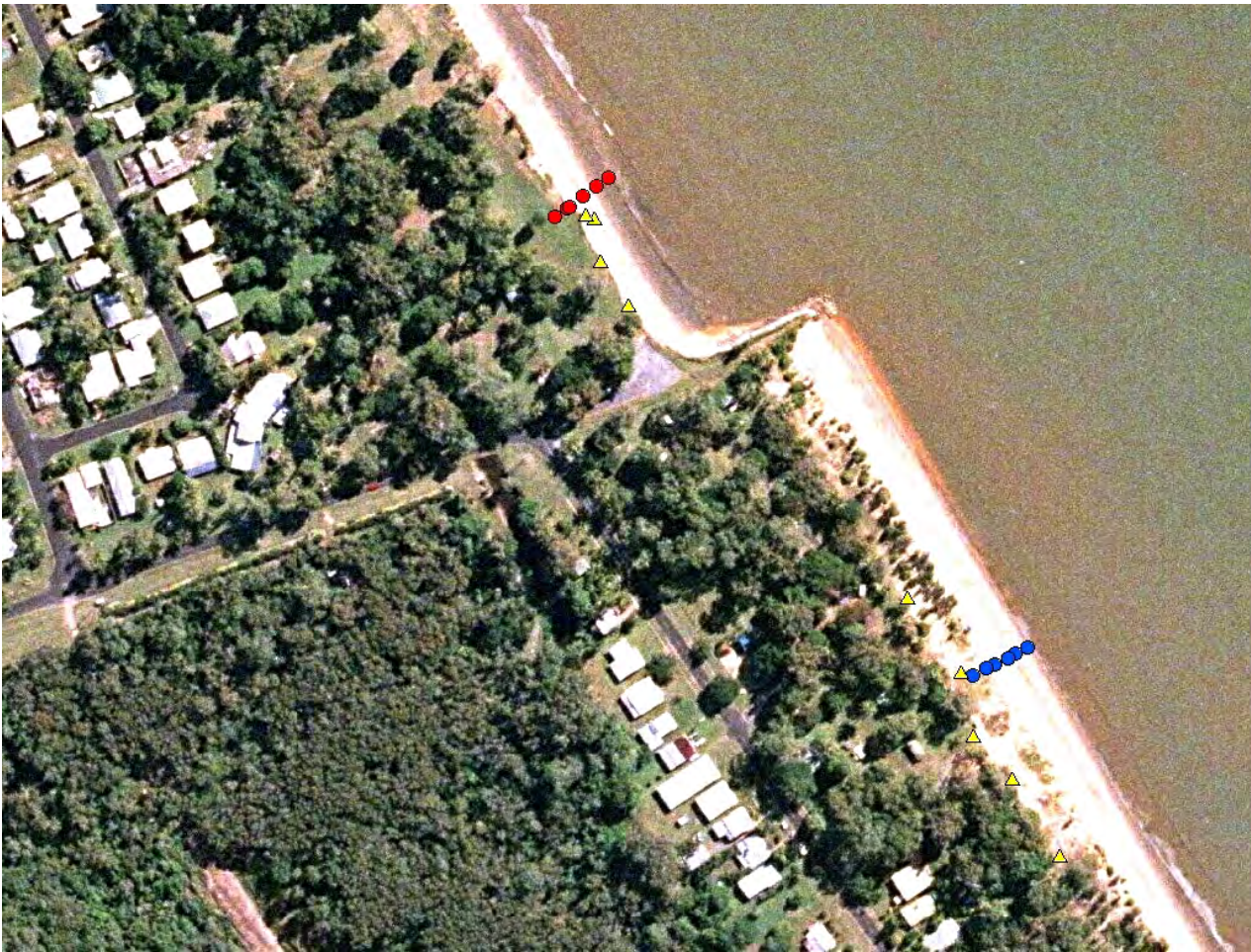
Figure 16: Bramston Beach surveyed beach profiles and debris lines (yellow triangles)
