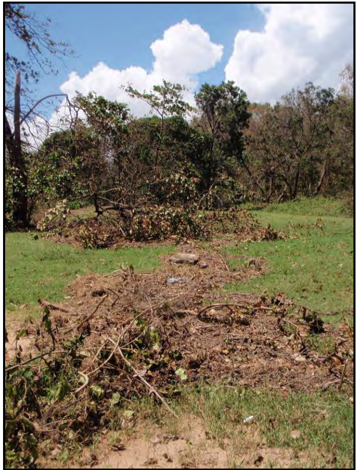
Photograph 42: Debris line used to survey storm tide inundation level (Source: DSITIA)
