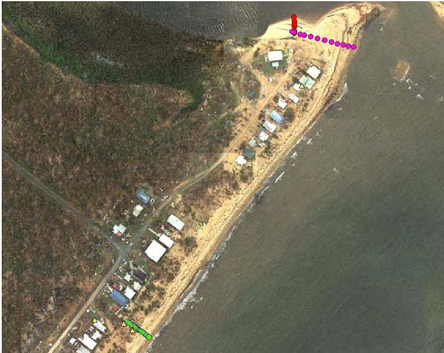
Figure 26: Hull Heads surveyed beach profiles and debris lines (yellow triangles)
