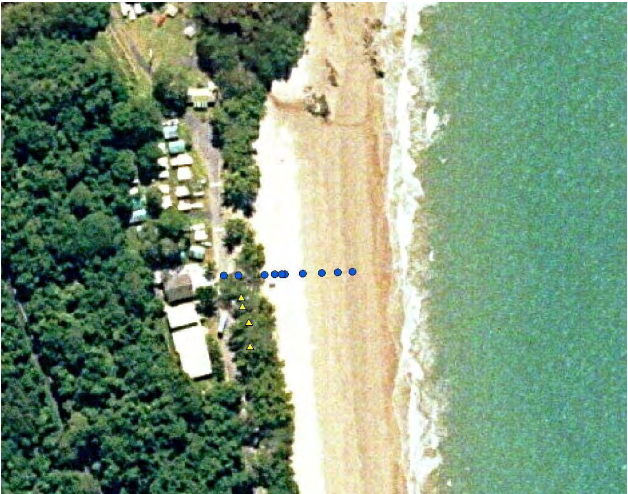
Figure 18: Etty Bay surveyed beach profiles and debris lines (yellow triangles)
