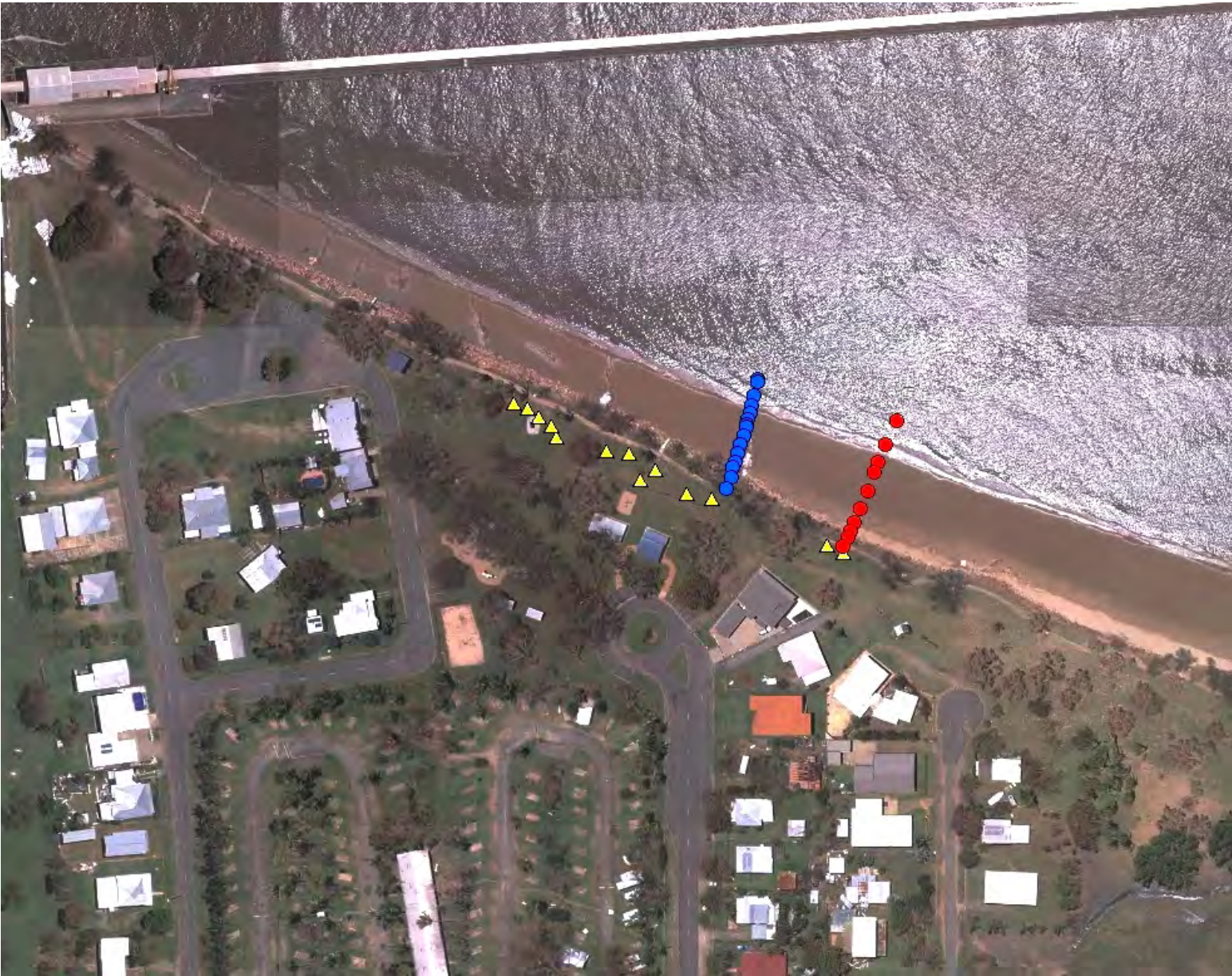
Figure 32: Lucinda surveyed beach profiles and debris lines (yellow triangles)
