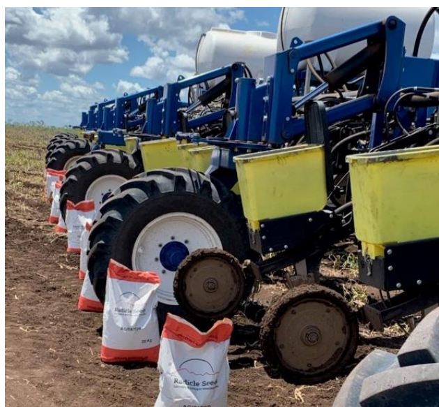
Figure 1: John Deere precision boxes with Precision Planting drive equipment. Each box holds 2 bags of sorghum seed. Photo: Shane Beil.
