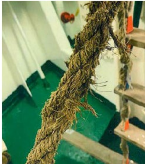
Photo 10: Frayed side rope.
