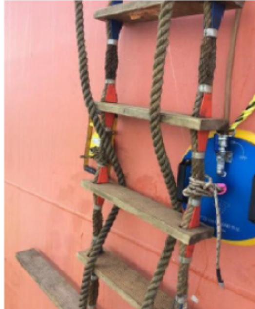
Manropes are to be tucked in line with the magnet/suction pad
