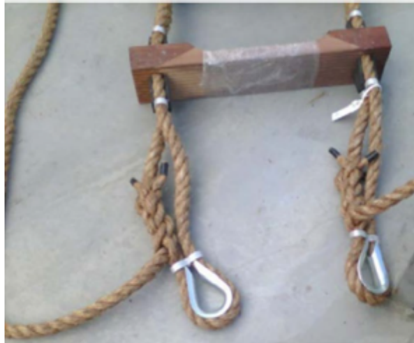
Photo 12: Example of non-compliant pilot ladder with splices in side ropes.
