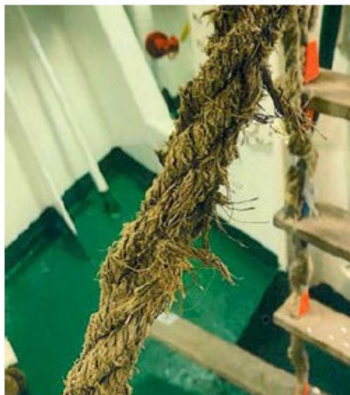
Photo 10: Frayed side rope.
