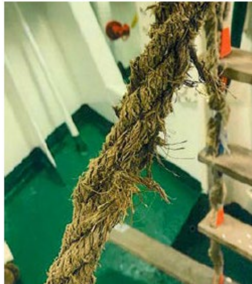
Photo 10: Frayed side rope.
