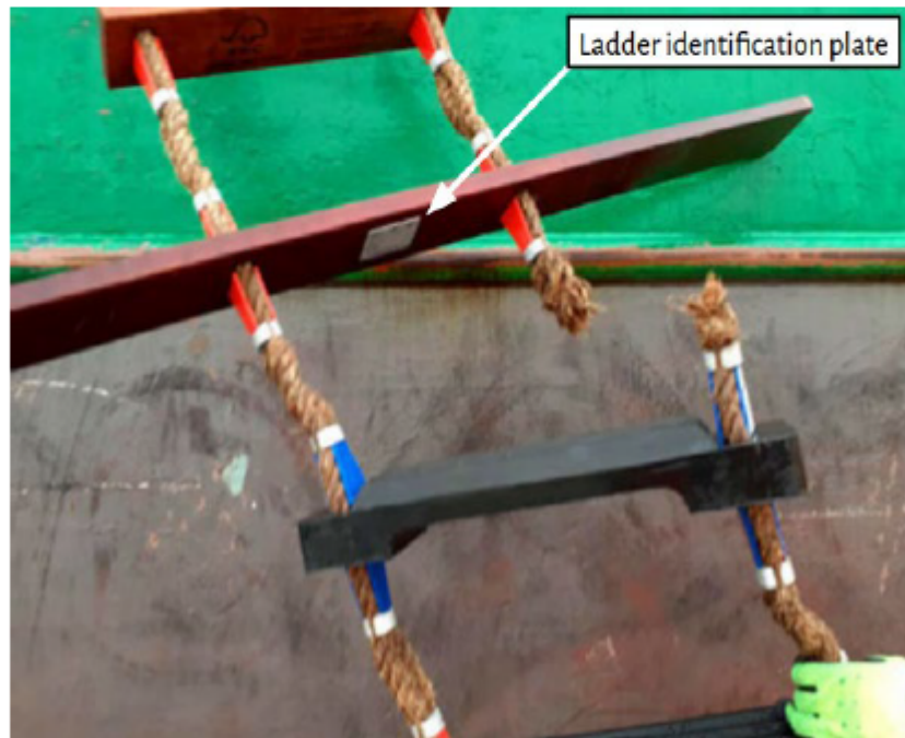
Photo 8: Pilot ladder where side ropes parted when in use (Reproduced with permission of the MAIB).
