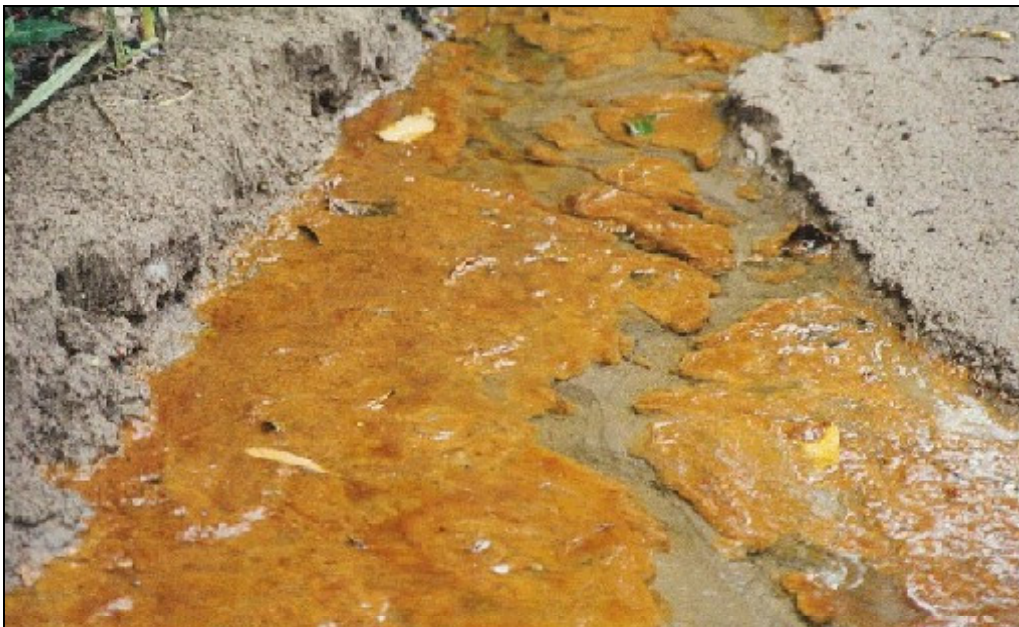
Plate 4. Iron oxides produced during oxidation of pyrite can choke drains
