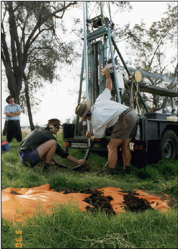
Plate 6. Vibro suction corer
