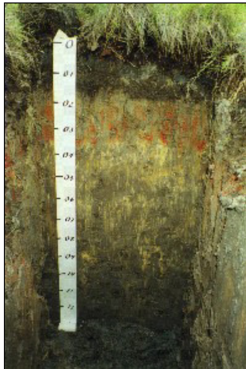
Plate 1. A typical acid sulfate soil profile. The oxidised actual acid sulfate soil layer is visible from 0.35–0.95 m, with jarositic (yellow-coloured) mottles present. The dark grey, unoxidised potential acid sulfate soil layer underlies the AASS layer.
