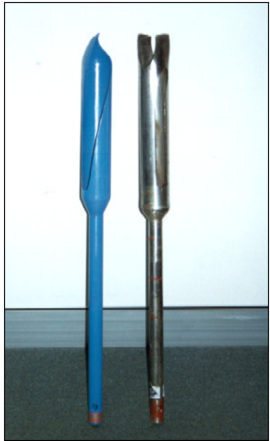
Plate 2. Dormer soil and Dormer sand augers
