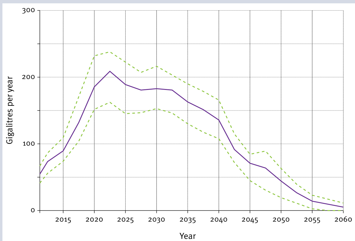
Figure 12.1 Estimated associated water production in the Darling Downs region—the middle line is the average estimate based on 99 simulations, while the dotted lines represent the 25th and 75th highest estimates
