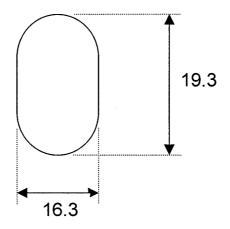
Cross Section of Lock Barrel
