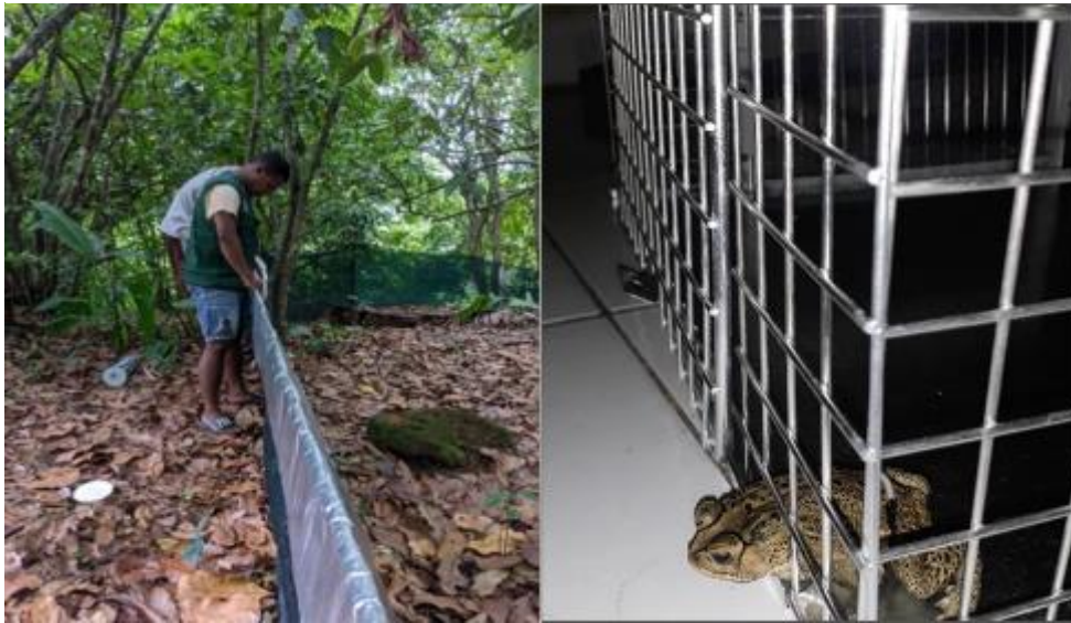
Figure 54 Left: Setting up an enclosed arena in Madagascar for field ABST trapping tests. Right: An ABST escaping from an unmodified Toadinator™ trap designed for cane toads.
