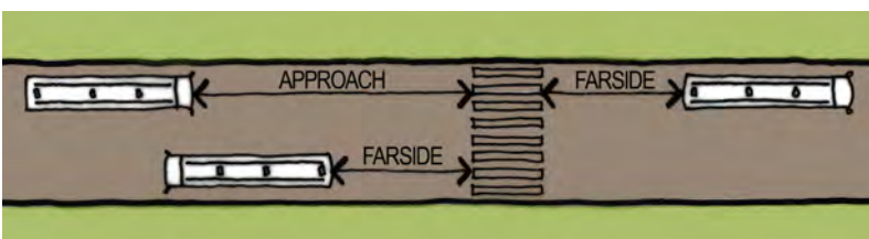
Figure 5.9 – Non-signalised pedestrian crossing
