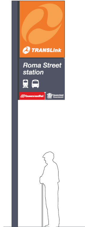
Figure 4.4 – Major station identification sign (8 or 9 meters high)
