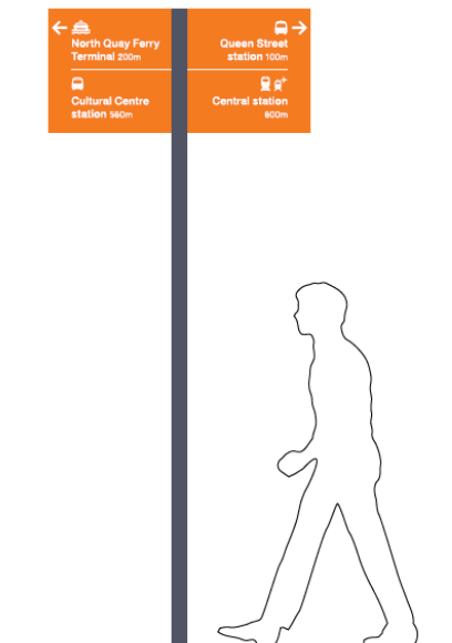
Figure 4.21 – External minor directional sign
