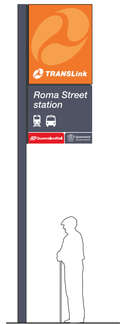
Figure 4.4 – Major station identification sign (8 or 9 metres high)
