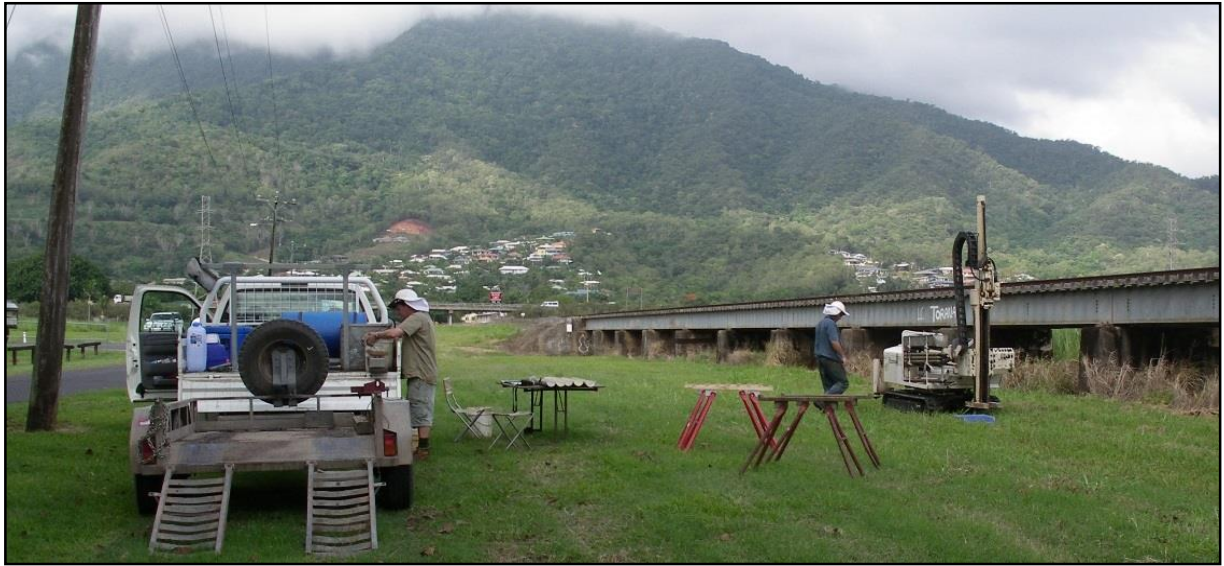
Plate 20. Site 203, Location: Ryan Wear Park, Kamerunga Rd, Map unit 5+, LiDAR elevation: 5.7m AHD, PASS depth: 6.7m, PASS elevation: -1.0m AHD.
