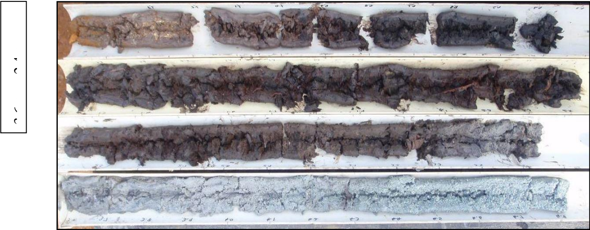
Plate 12. Site 262 Soil Profile to 4.8m
