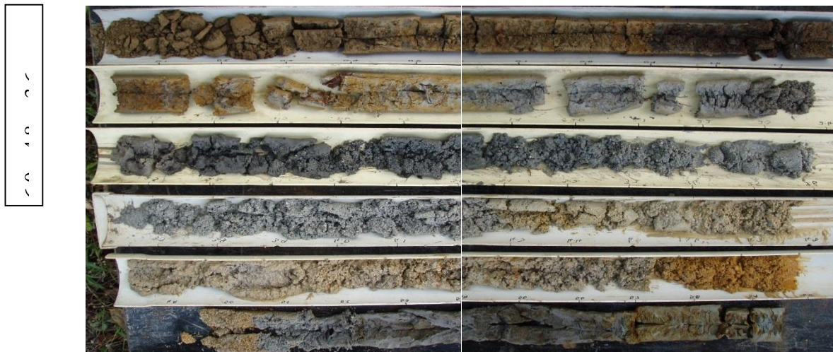
Plate 38. Site 178 Soil Profile to 7.2m
