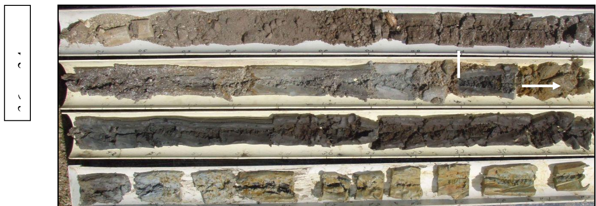
Plate 25. Site 183 Soil Profile to 4.8m
