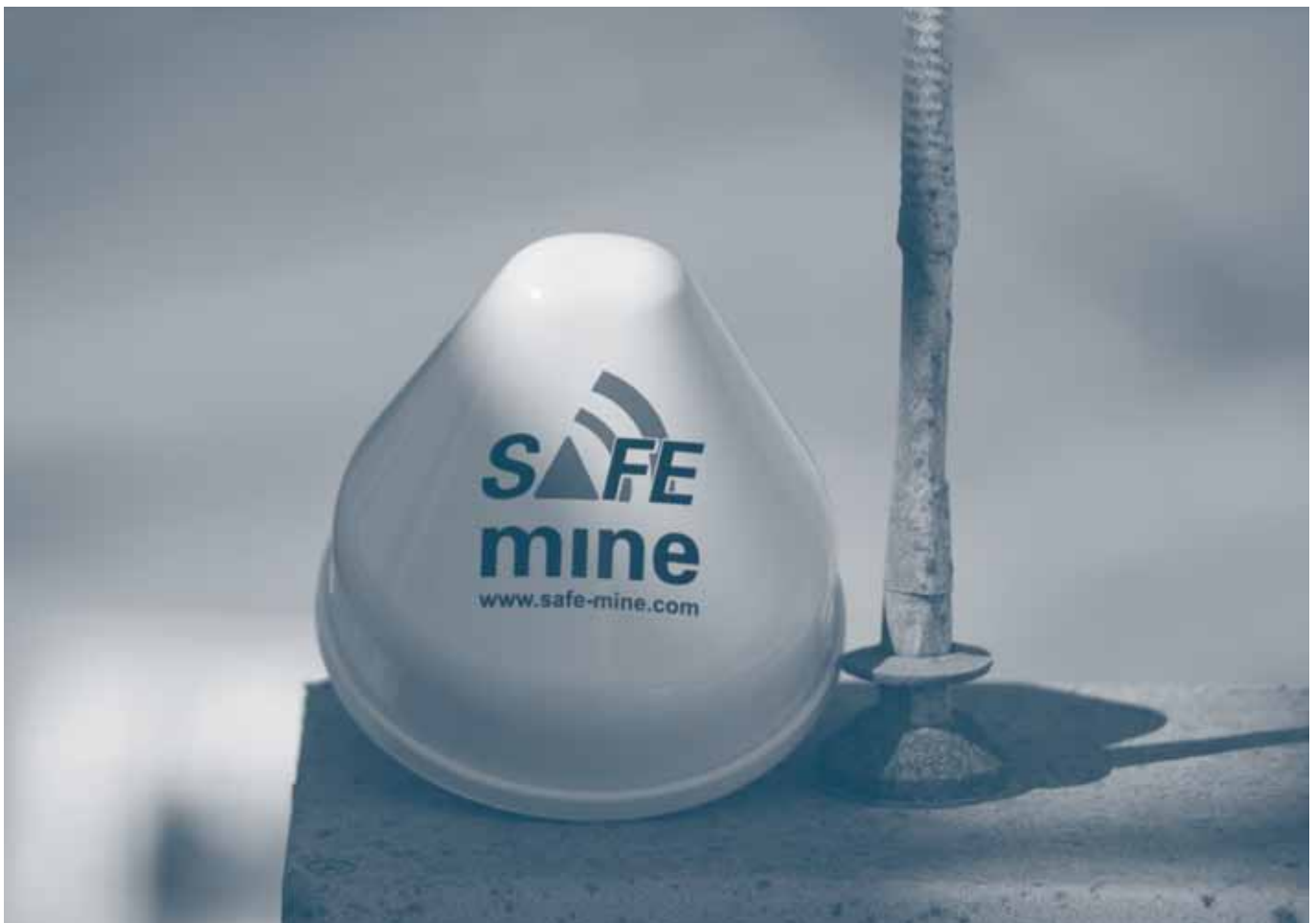
Safe mine — proximity detection system, Meandu Mine Photo: DNRM
