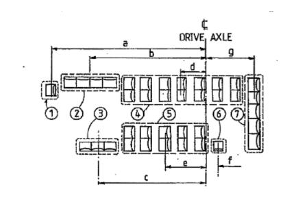
Determine the seated loading factor separately for those seats in front of and those behind the drive axle line, by multiplying the number of seating positions by the longitudinal distance from the drive axle line and adding to get a sub-total.
