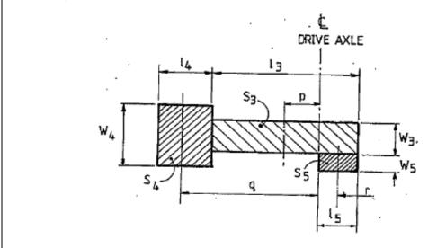
Calculate the maximum standing capacity in the front section by summing the total standing area and multiplying by 6.25 persons/m². Take the nearest whole number less than this value for maximum standing capacity. The nominated capacity must not be more than this.
