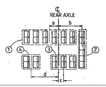
Determine the seated loading factor separately for those seats in front of and those behind the rear axle line, by multiplying the number of seating positions by the longitudinal distance from the rear axle line and adding to get a sub-total.
