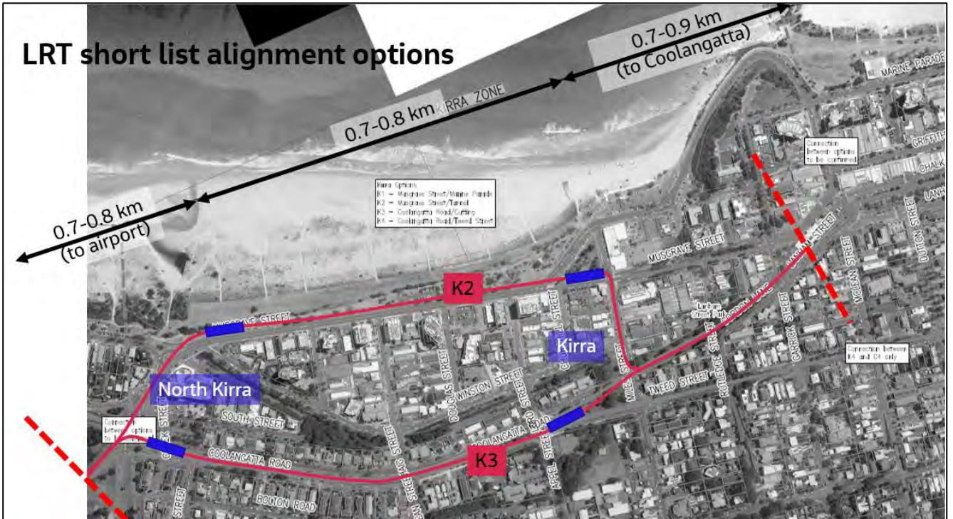
Figure 7-14: Kirra short list alignment and station options – high level design (Aerial image: Metromap, 2020)
