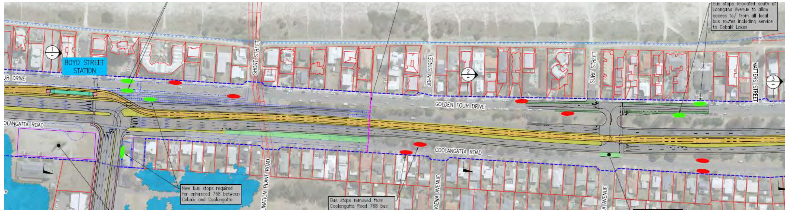
Figure 7-6: Alignment Option B2-3 design (between and including Boyd Street and Loongana Avenue)
