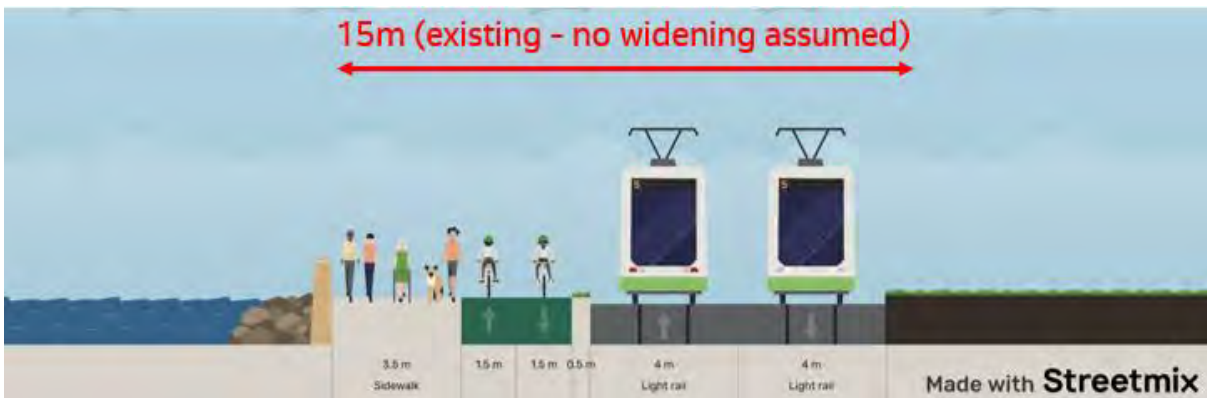
Figure 6-13: Marine Parade – Alignment K1 indicative cross section
