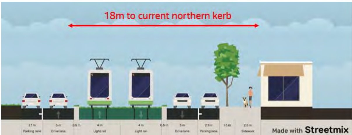
Figure 6-12: Musgrave Street – Alignment K1/K2 indicative cross section
