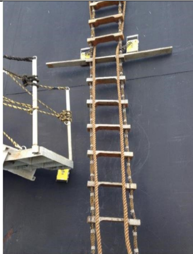
Magnets must be 1.5 meters above combination ladder platform
