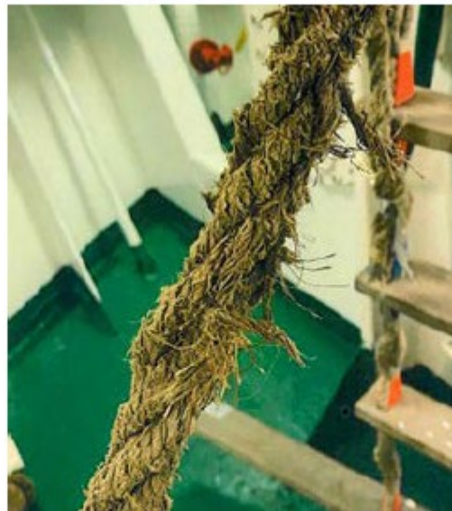
Photo 10: Frayed side rope.
