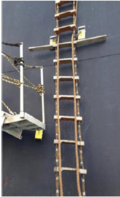
Magnets must be 1.5 metres above combination ladder platform
