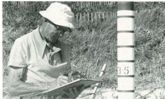
COPE observer at Burleigh Heads, Bill Patterson records the level of the beach at the COPE reference pole. The graduations on the pole are also used to measure the cross-section shape of the beach.
