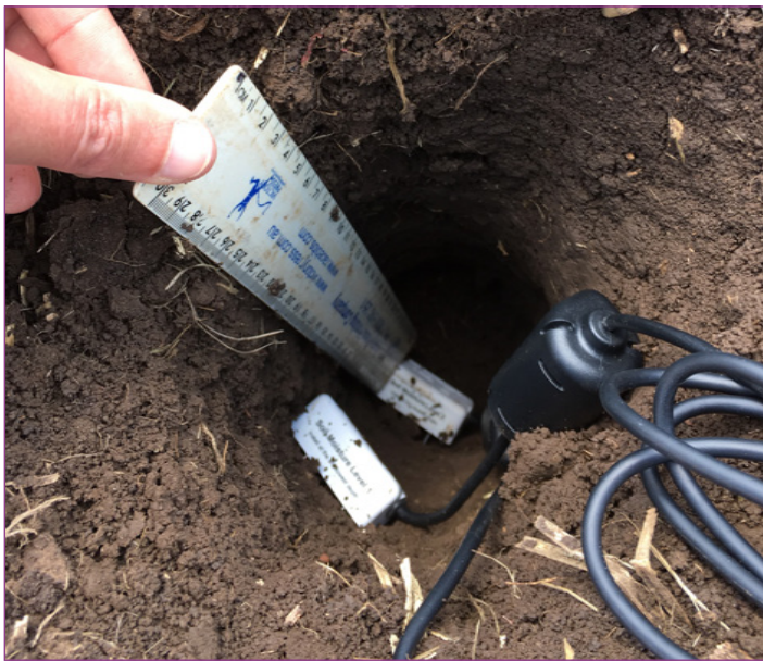
Figure 2. The sensors are placed at 15 cm and 30 cm depths to measure the moisture at two levels in the corn root zone.
