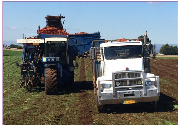
Figure 1. Twin row ASA-lift™ carrot harvester with yield monitoring technology. The load cells are located in part of the elevator that supplies the bunker. The collection of accurate yield data is dependent on a good harvester operator following protocols for yield monitor operation and taring.
