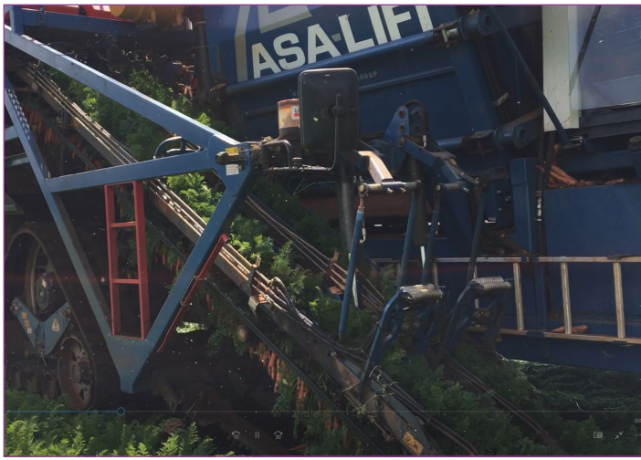
Figure 1. Twin row ASA-lift™ carrot harvester with yield monitoring technology. The load cells are located in part of the elevator that supplies the bunker. The collection of accurate yield data is dependent on a good harvester operator following protocols for yield monitor operation and taring.
