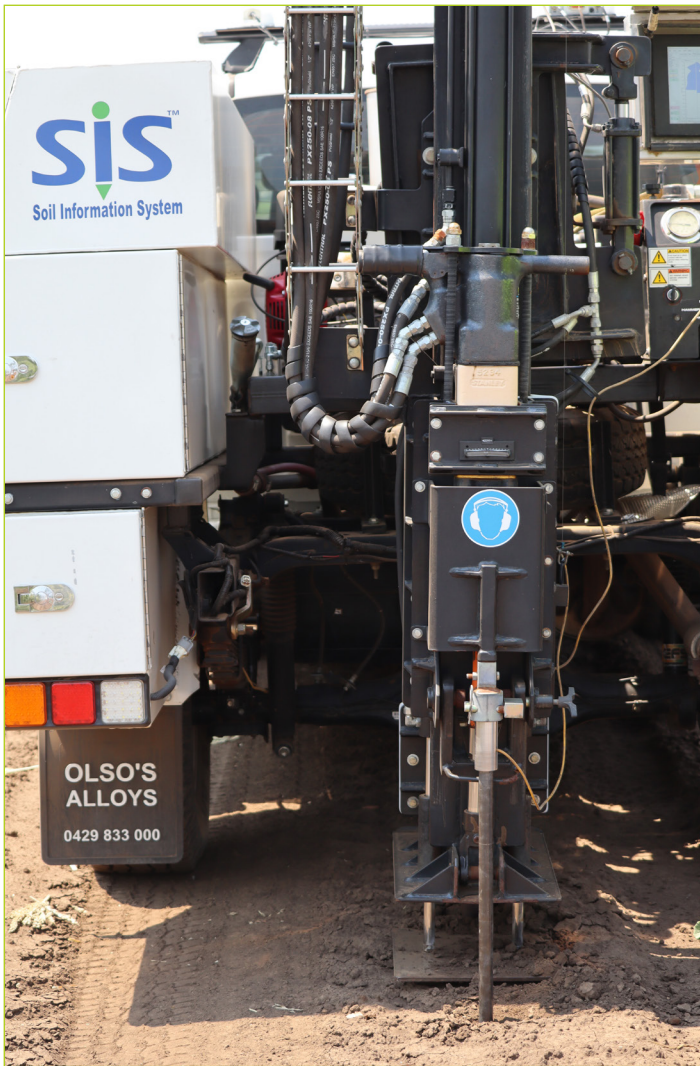
Figure 6. SIS™ rig with sampling cores. Source: DAF
