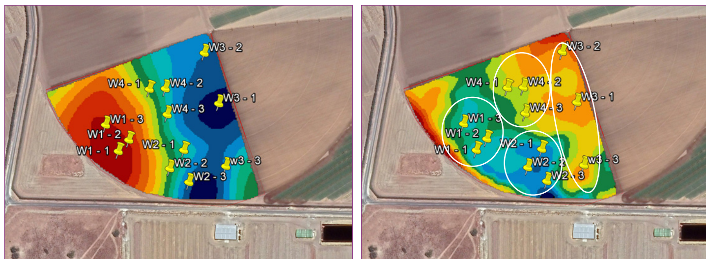
Figure 6. Location of yield sampling points in the field relative to both the elevation (left) and EM38 (right) maps. Circles indicate the approximate zones with three yield samples from each of these areas.
