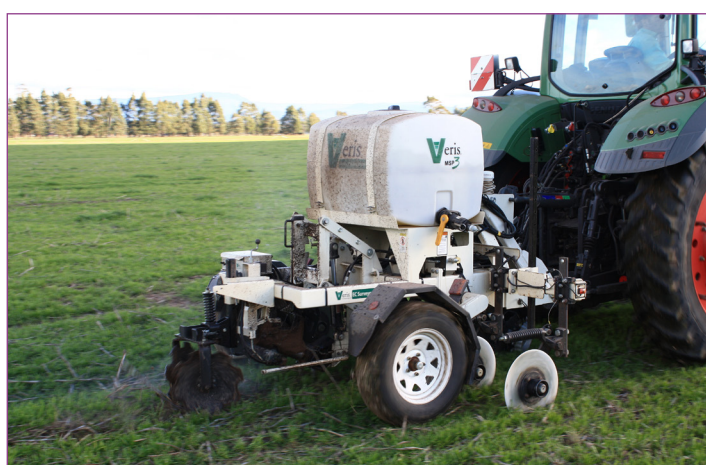
Figure 1. Veris® soil mapping rig uses on-the-go soil sensors with geo-referencing to create a soil map of an area.
