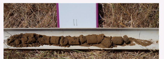
Figure 2. Left: Soil type areas identified from EM38 soil mapping. Dark blue areas indicate higher EC and contained clay, red areas were lower EC and were predominantly sand. Right: Soil cores showing soil cores from ground-truthing.
