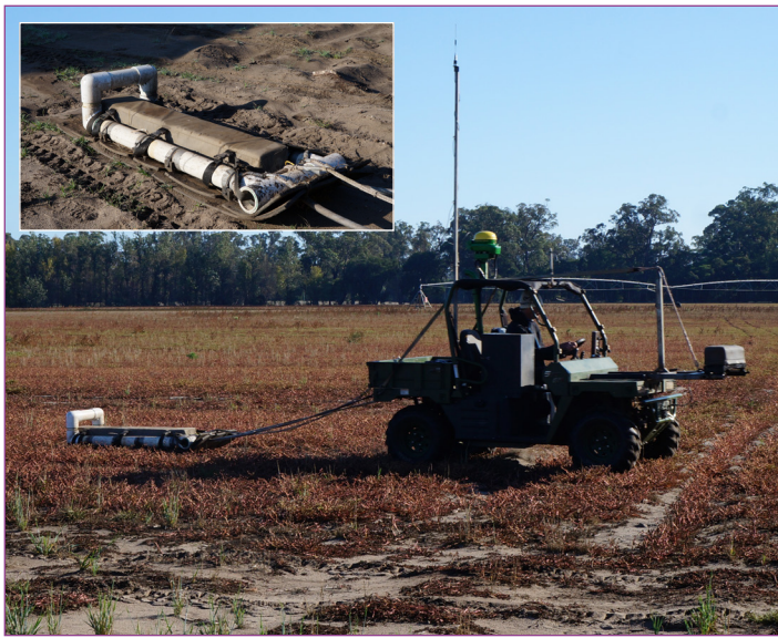
Figure 1. EM38 Soil mapping (left and inset) and drone taking off for plant counts and crop sensing (right).
