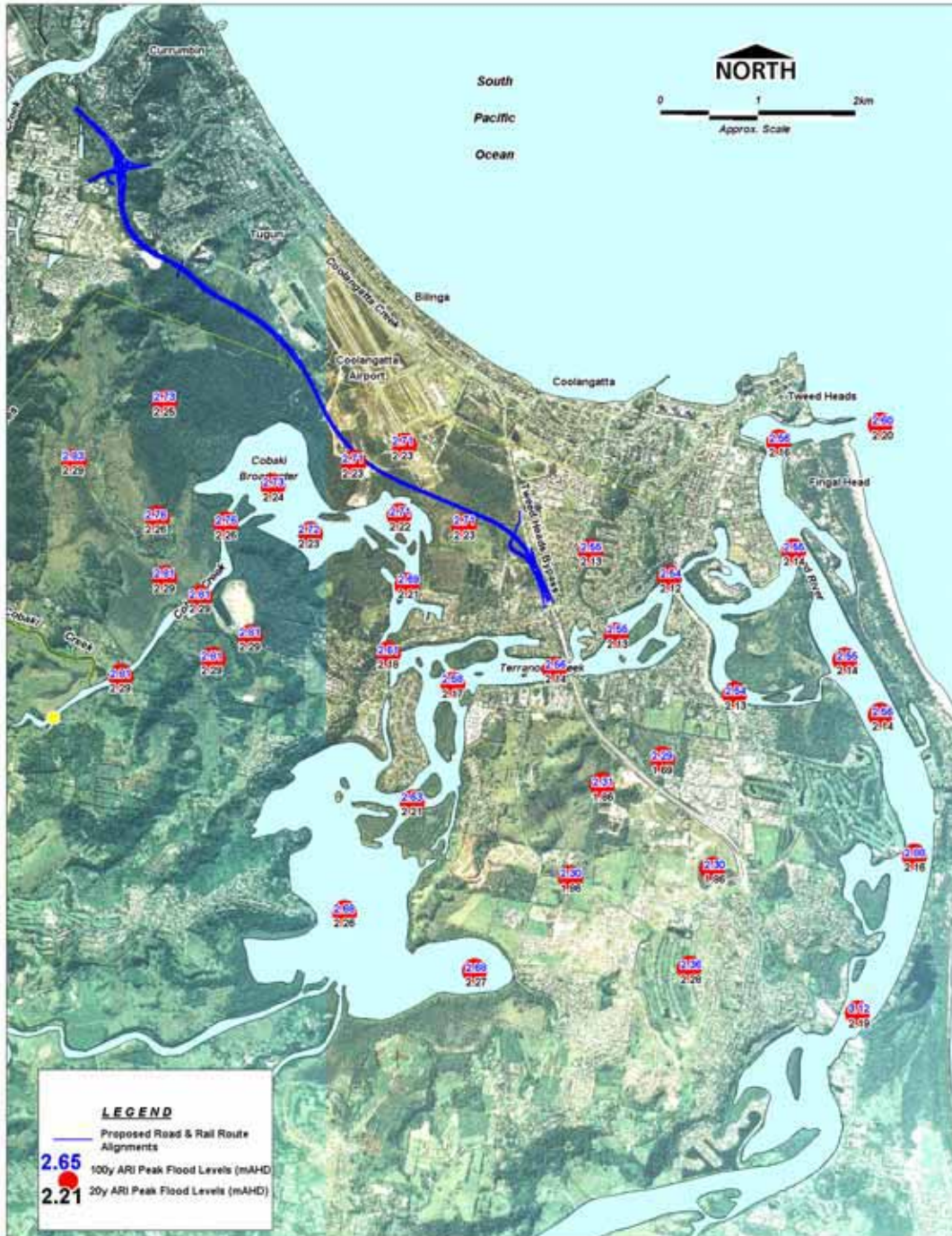
Figure 3.10: Existing Peak Flood Levels - Tweed River
