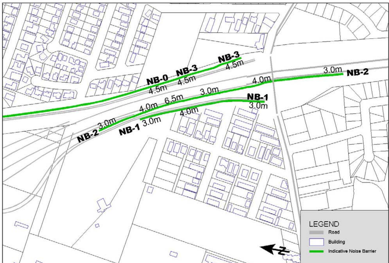
Figure 11.2b: NSW Indicative Noise Barrier Locations (b)
