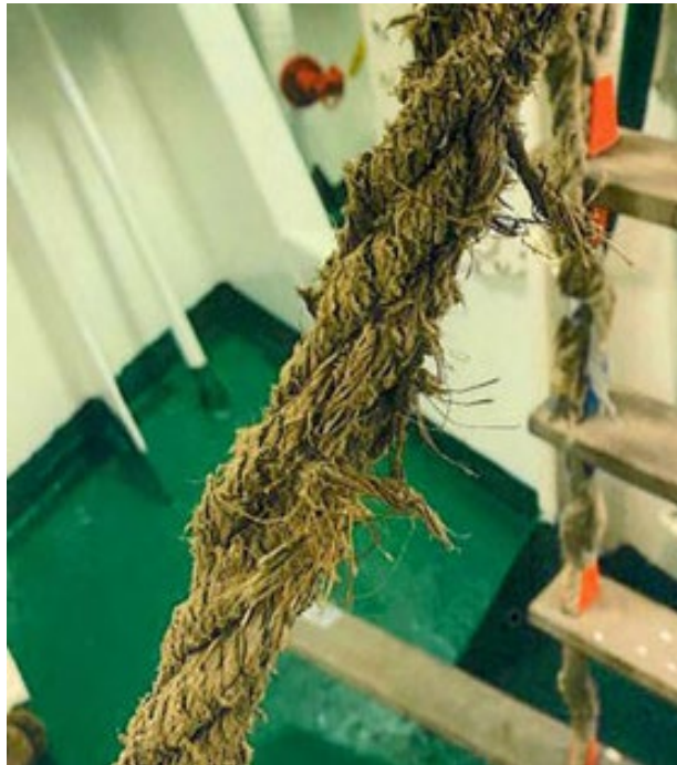
Photo 10: Frayed side rope.
