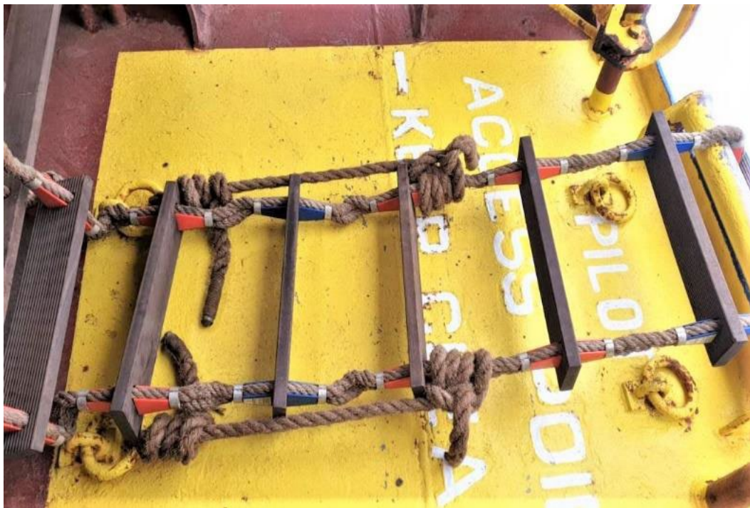
Photo 7: Rolling hitch knots being used to secure pilot ladders to approved main deck strong points (Reproduced with permission from Fremantle Ports).
