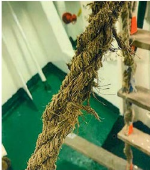
Photo 10: Frayed side rope.
