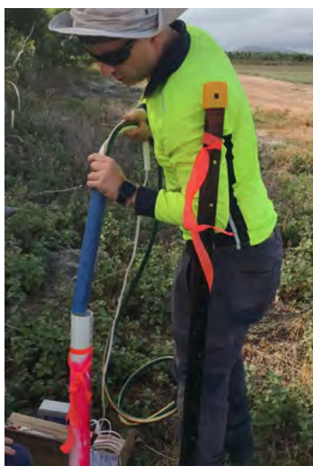
Figure 19: Groundwater sampling using a water pump in a piezometer.
