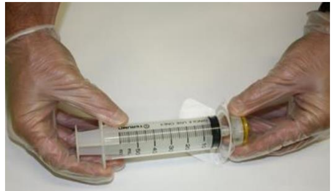
Figure 1: Connect the 0.45 µm syringe filter to the syringe (photo: from DES. 2018. Monitoring and Sampling Manual: Environmental Protection (Water) Policy. Brisbane: Department of Environment and Science Government).
