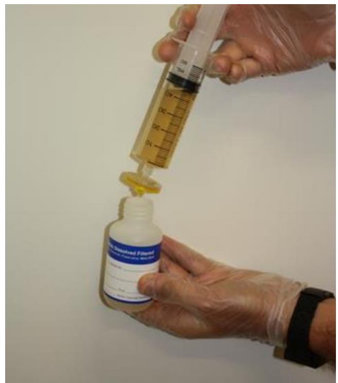
Figure 2: Discharge the water sample into the bottle (photo: from DES. 2018. Monitoring and Sampling Manual: Environmental Protection (Water) Policy. Brisbane: Department of Environment and Science Government).
