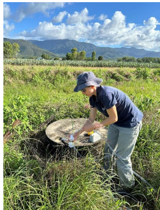
Figure 4: Fill the sample bottle with the water being pumped out of a piezometer or well.
