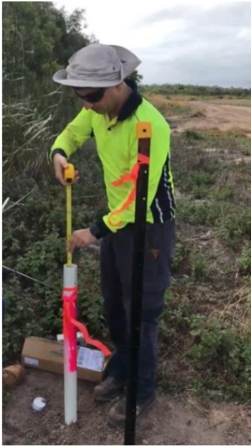
Figure 1: Put the tape measure into the piezometer until it touches the water. Record the height from the water to the top of the PVC pipe.
