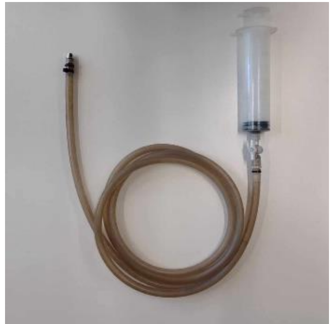
Figure 2: A tube attached to a syringe can be used to collect a groundwater sample.
