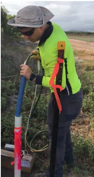
Figure 3: A water pump inserted into the piezometer can be a quick and easy way to purge the piezometer and collect a groundwater sample.
