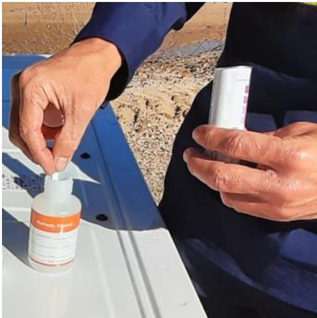
Figure 1: Immerse the end of the nitrate test strip in the sample for a second.
