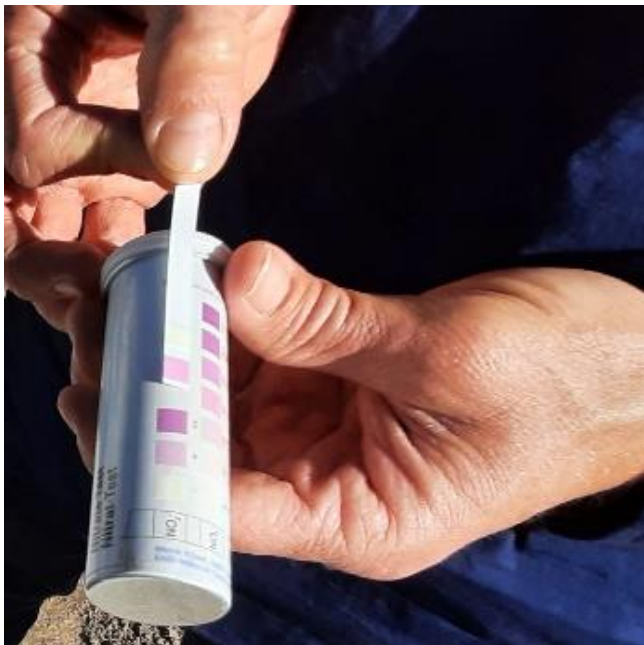
Figure 2: Compare the strip with the colour scale on the container.
