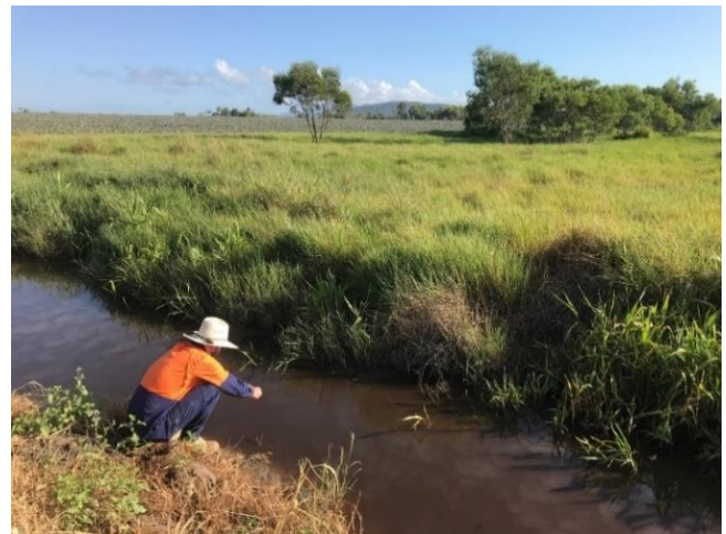
Figure 2: A sample can also be collected by hand in smaller drains like this.
