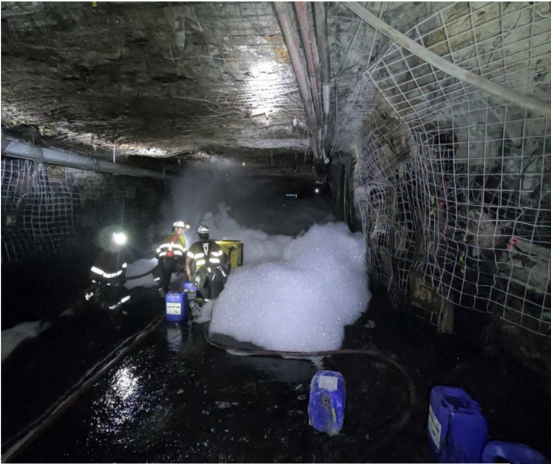
Figure 5 Photo shown to firefighting responders at incident site using Turbex foam generator
