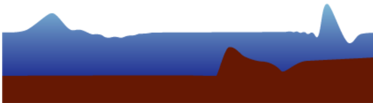
(c) Deep water wave travels faster, whilst shallow wave shoals.
