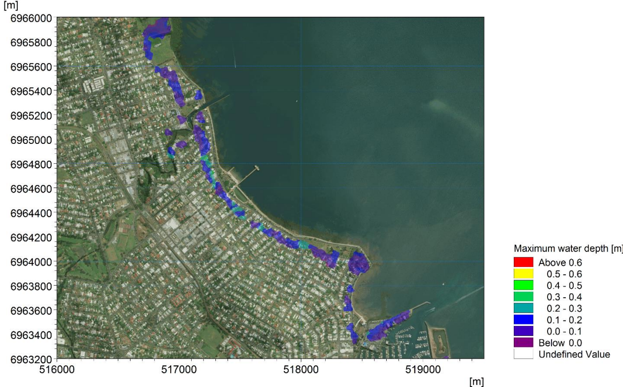
Figure 31 - Additional inundation extent and depths for Scenario 1 (scouring of North and South Passage to RL -5m).
