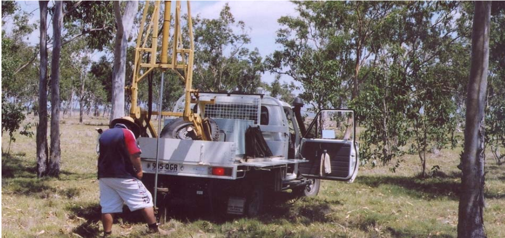
Figure 3. Push tube sampling, elevated plain, Pelican Creek.
