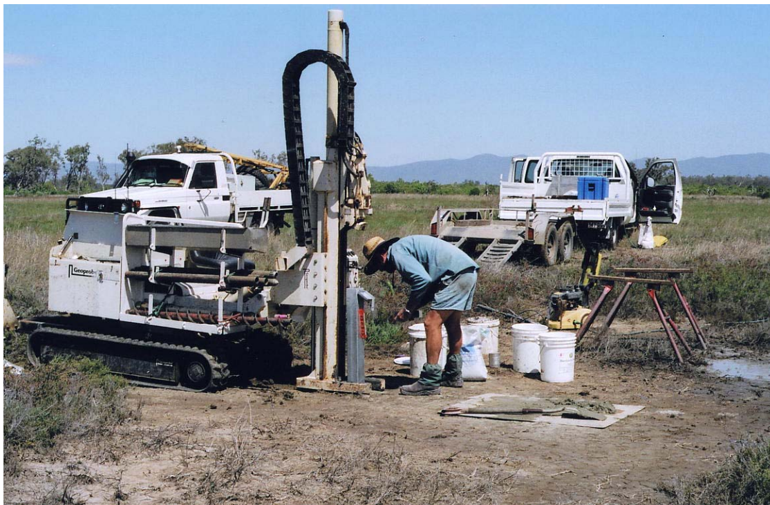
Figure 13. Installation of piezometer F, Eight Mile Creek.
