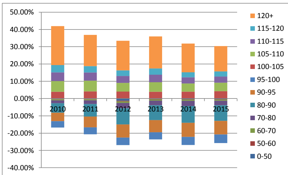
Figure 14 Estimated fractions of casualty crashes attributable to each speed range on 100km/h limit roads. Negative values indicate fraction of crashes saved by speeds below limit.
